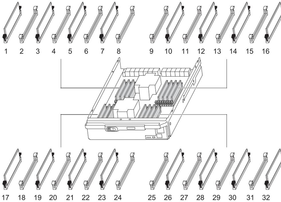
3. Eject the DIMM from its slot by slowly pushing apart the two DIMM ejector tabs on either side of the DIMM, and then slide the DIMM out of the slot.
