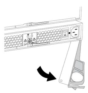
6. Use the cam handle to slide the power supply out of the disk shelf.
