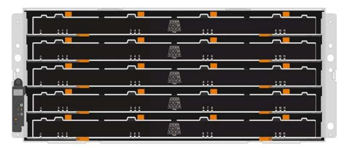
• The following illustration shows how the drives are numbered from 0 to 11 in each drive drawer within the shelf.
