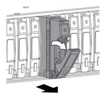
6. Slide out the disk drive slightly to allow the disk to safely spin down, and then remove the disk drive from the disk shelf.
