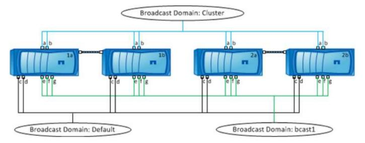
A failover group of the same name and with the same network ports as each of the broadcast domains is created automatically. This failover group is automatically managed by the system, meaning that as ports are added or removed from the broadcast domain, they are automatically added or removed from this failover group.
