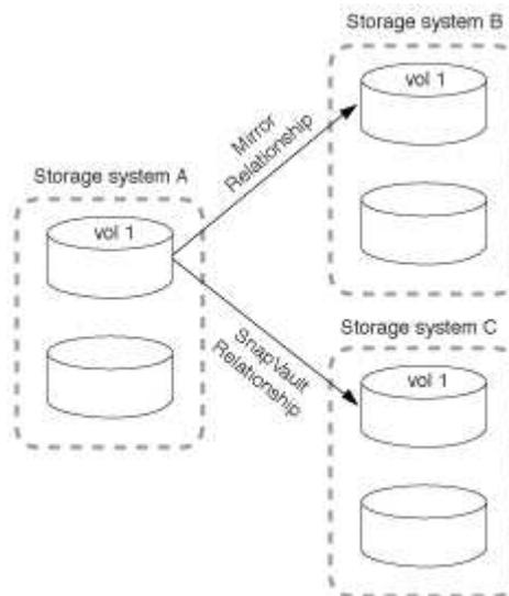
Starting with ONTAP 9.5, you can have fan-out deployments with SnapMirror Synchronous relationships; however, only one relationship in the fan-out configuration can be a SnapMirror Synchronous relationship, all the other relationships from the source volume must be asynchronous SnapMirror relationships.
