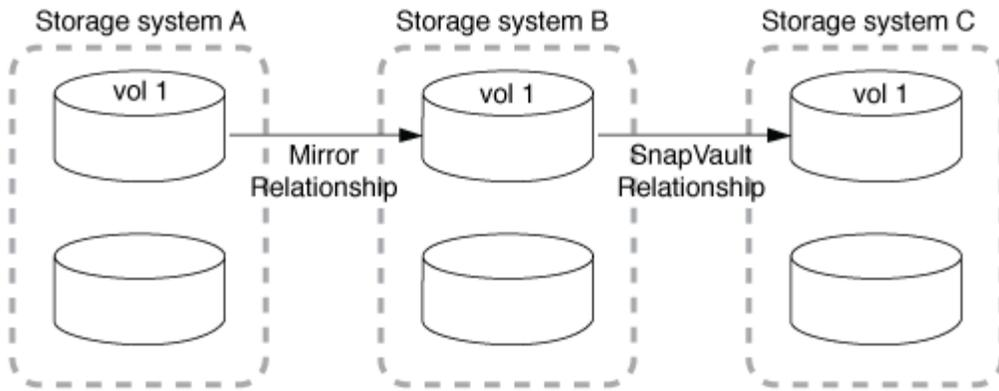
Vault-mirror and, starting with ONTAP 9.2, vault-vault cascade deployments are also supported:
