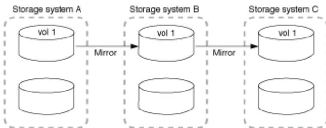
A mirror-vault cascade deployment consists of a chain of relationships in which a source volume is mirrored to a secondary volume, and the secondary volume is vaulted to a tertiary volume.
