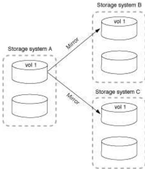
A mirror-vault fan-out deployment consists of a source volume that has a mirror relationship to a secondary volume and a SnapVault relationship to a different secondary volume.
