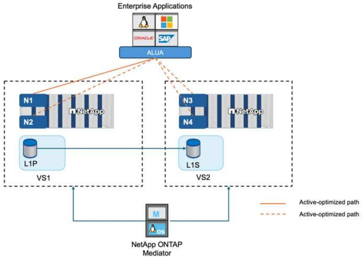
TAF operates in two modes: Automated Failover and Automated Failover Duplex. With Automated Failover, reads and writes are serviced only by the primary volume, therefore, I/Os issued to the mirror copy (which cannot service writes on its own) are proxied to the primary copy. With Automated Failover Duplex, both the primary and secondary copies can service I/Os so no proxy is necessary.
