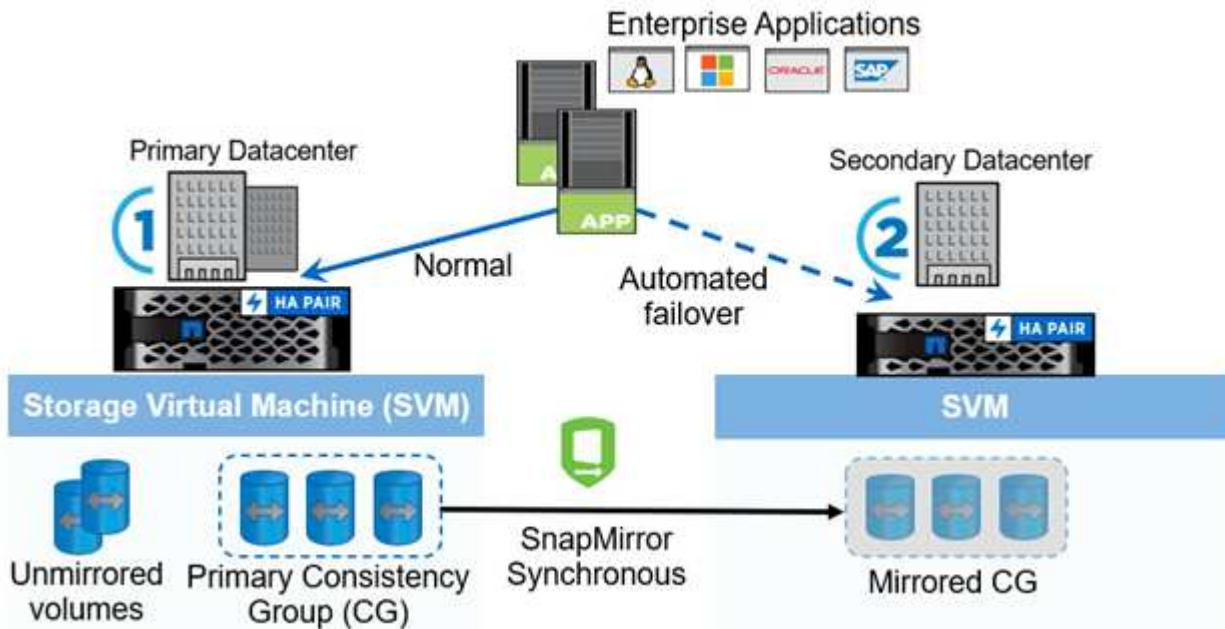
The diagram shows an enterprise application that is hosted on a storage VM (SVM) at the primary data center. The SVM contains five volumes, three of which are part of a consistency group. The three volumes in the consistency group are mirrored to a secondary data center. In normal circumstances, all write operations are performed to the primary data center; in effect, this data center serves as the source for I/O operations, while the secondary data center serves as a destination.
