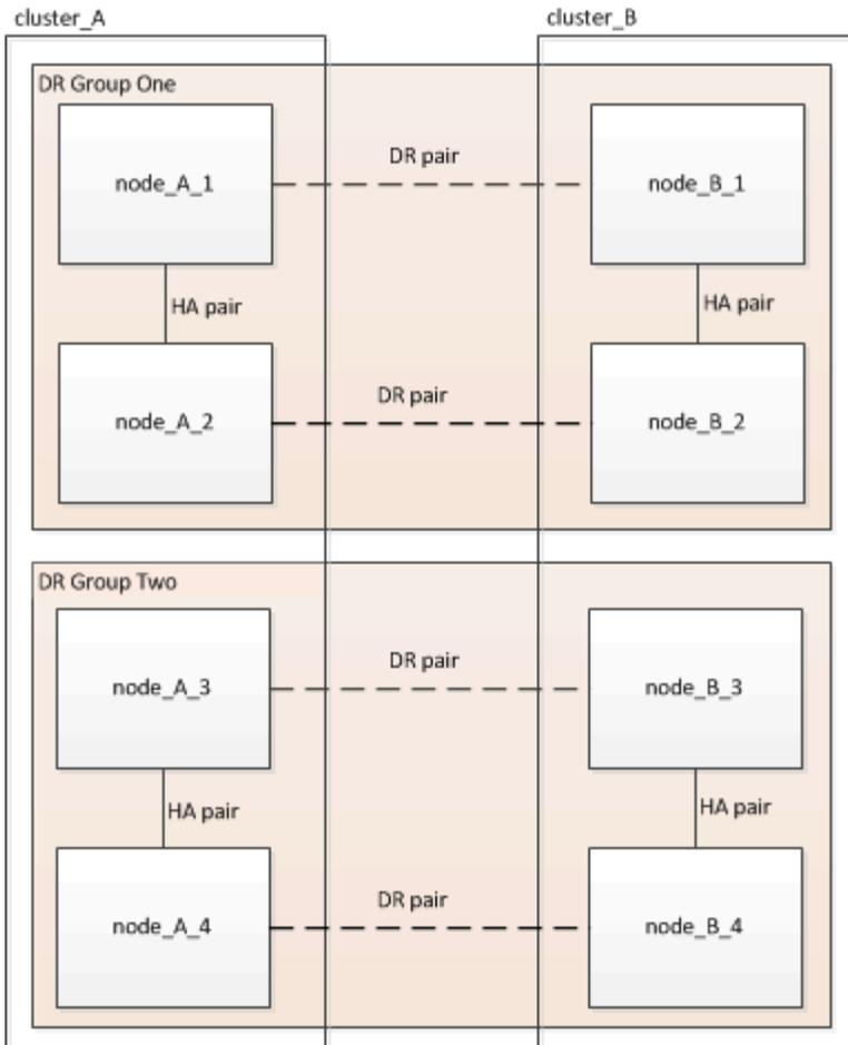
The MetroCluster software update procedure involves upgrading or downgrading one DR group at a time.
