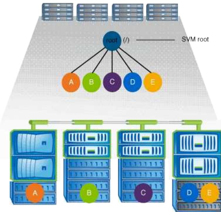
For example, a typical volume junction configuration with the above namespace architecture might look like the following configuration, where there are five insertion points to the root volume of the SVM, with each insertion point representing a path to one volume.
