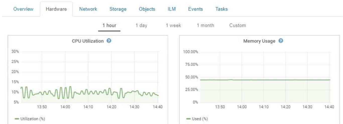
To display a different time interval, select one of the controls above the chart or graph. You can display the information available for intervals of 1 hour, 1 day, 1 week, or 1 month. You can also set a custom interval, which allows you to specify date and time ranges.
