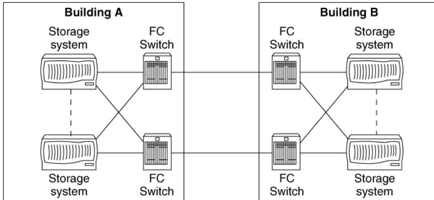
The storage systems in each building are arranged in an HA pair. An HA pair removes single points of failure and provides a more practical, fault-tolerant setup.
