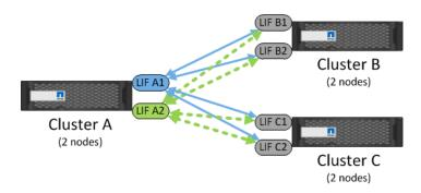
If you do want a cluster peer relationship between two remote clusters in addition to the fan-in or fanout configuration, then use the concept of *pair-wise full-mesh* connectivity to create an intercluster network between them.
