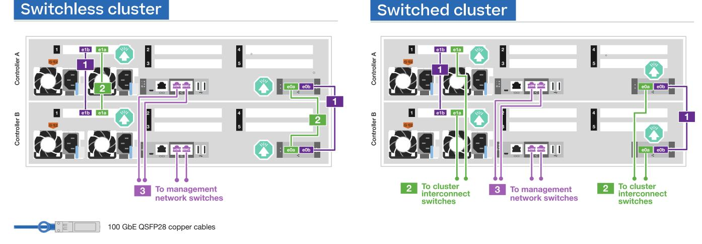
Connect port e1b to port e1b and port e0b to port e0b (HA interconnect only).
