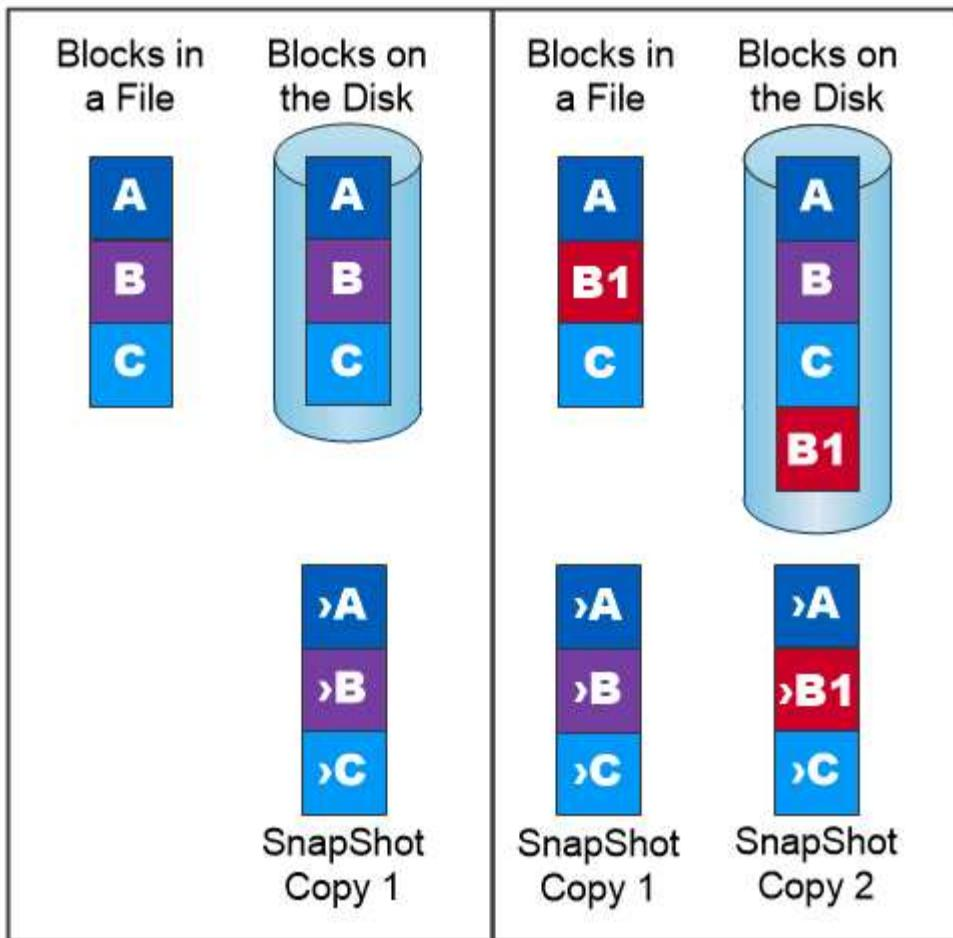
*A Snapshot copy records only changes to the active file system since the last Snapshot copy.*
