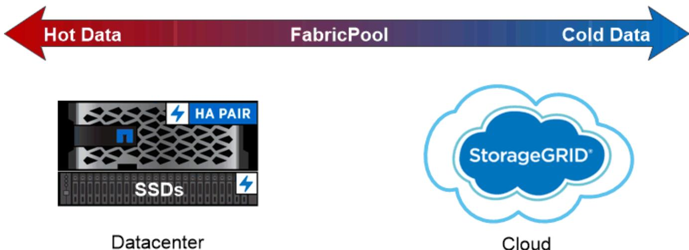
*You can use a FabricPool to tier data with different access patterns, deploying SSDs for frequently accessed “hot” data and object storage for rarely accessed “cold” data.*
