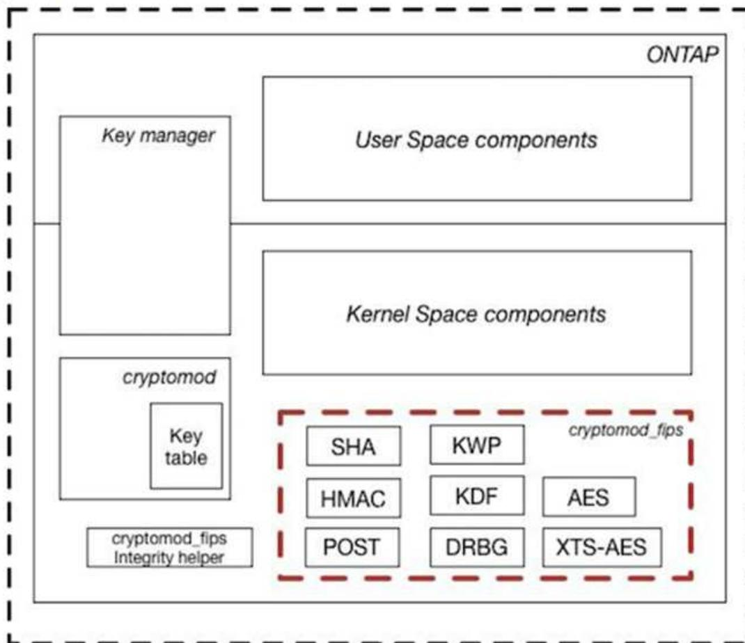
Figure 1 - Block Diagram
