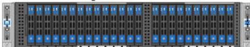
H410S storage nodes in a four-node chassis
