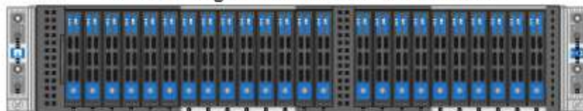
H410S storage nodes in a four-node chassis
