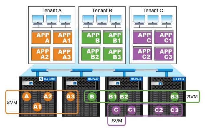
Service providers use SVMs in multitenant environments to isolate tenant data and simplify chargeback.
