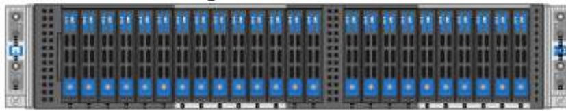
H410S storage nodes in a four-node chassis
