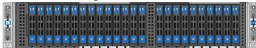
H410S storage nodes in a four-node chassis
