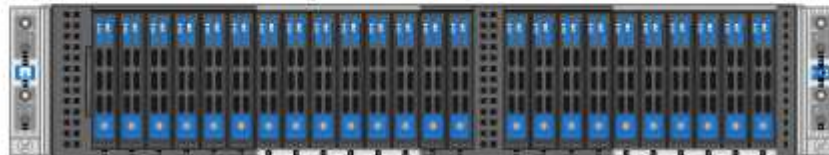
H410S storage nodes in a four-node chassis
