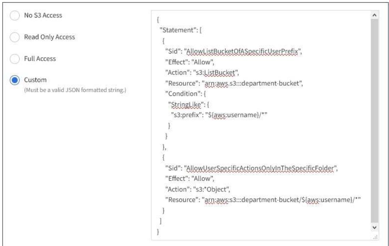
The screenshot shows the AWS IAM console interface for configuring a group policy. On the left side, there are four radio button options: 'No S3 Access', 'Read Only Access', 'Full Access', and 'Custom'. The 'Custom' option is selected, and a note below it says '(Must be a valid JSON formatted string.)'. On the right side, there is a text area containing a JSON policy document. The JSON is as follows:
