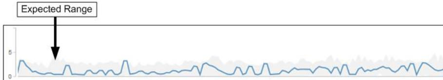
In this example, the latency for a volume has an expected range, in gray, of 0 milliseconds per operation (ms/op) at its lowest and 5 ms/op at its highest. If the actual latency, in blue, suddenly increases to 10 ms/op, due to an intermittent spike in network traffic or contention on a cluster component, it is then above the expected range and has exceeded the performance threshold.
