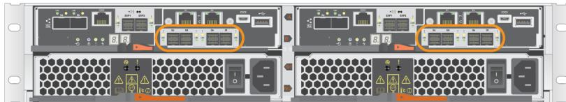
The following figures show an E5760 controller shelf before and after a HIC upgrade. The two HICs in the first figure have four SFP+ (optical) host ports each, and the two HICs in the second figure have four SAS ports each.
