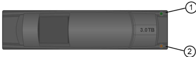
The following figure shows the LEDs on the drives in the E2824 controller shelf and the DE224C drive shelf:
