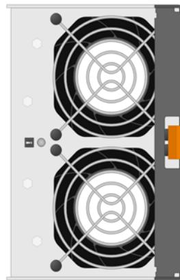
The following figure shows the back of a DE460C shelf with two fan canisters:
