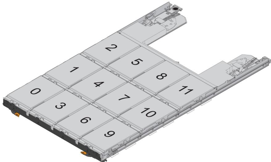
**Attention: Possible loss of data access** – Make sure to record the exact location of each drive before removing it.
