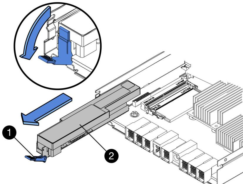
1 Battery release latch      2 Battery
