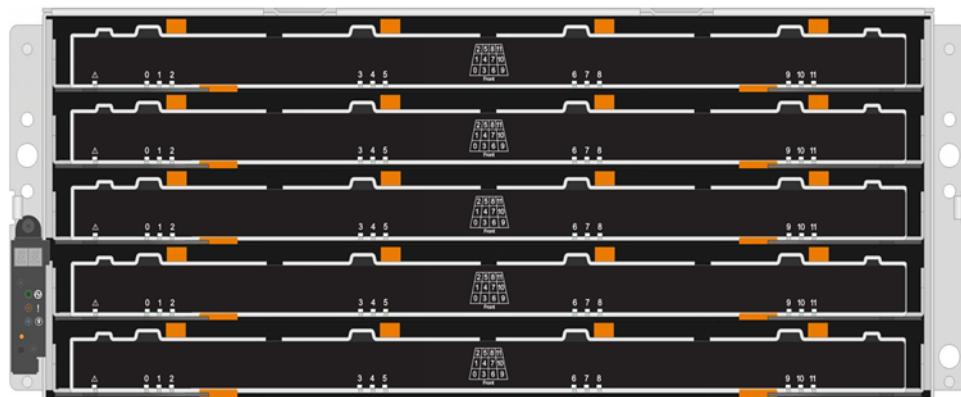
For both an E5760 controller shelf drawer and a DE460C drive shelf drawer, drives are numbered from 0 to 11 in each drive drawer within the shelf.
