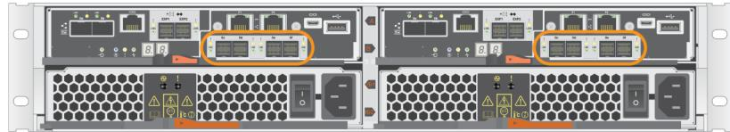
The following figures show an E5760 controller shelf with two controller canisters before and after adding a HIC into each controller.
