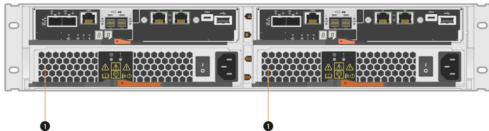
1 Controller shelf with two power supplies (power-fan canisters) below the controller canisters.
