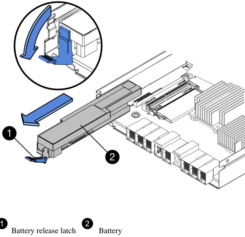
1 Battery release latch    2 Battery
