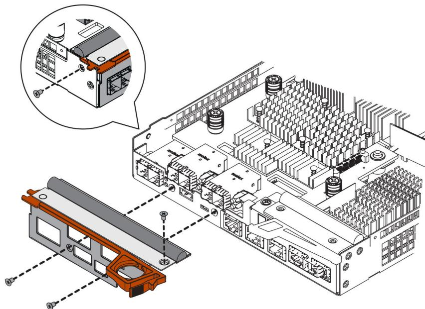
3. Align the three thumbscrews on the HIC with the corresponding holes on the controller, and align the connector on the bottom of the HIC with the HIC interface connector on the controller card. Be careful not to scratch or bump the components on the bottom of the HIC or on the top of the controller card.
