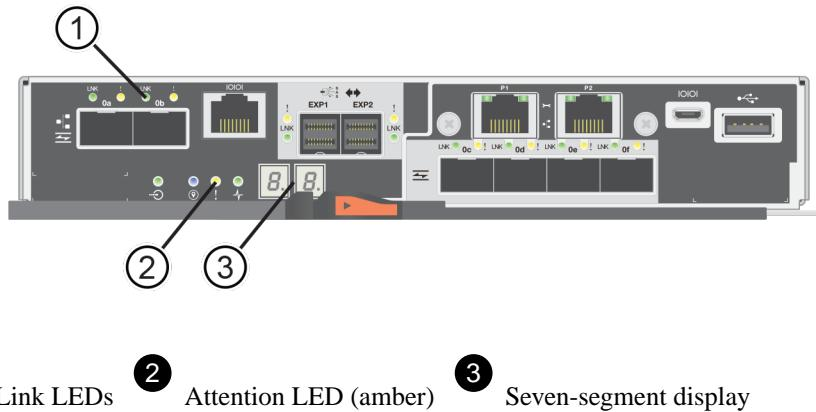
3. From SANtricity System Manager, confirm that the controller's status is Optimal. If the status is not Optimal or if any of the Attention LEDs are on, confirm that all cables are correctly seated, and check that the HIC and the controller canister are installed correctly. If necessary, remove and reinstall the controller canister and the HIC.
