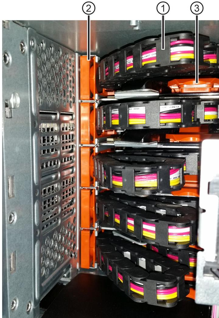
**1** Cable chain   **2** Vertical connector (connected to midplane)
