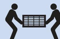
To reduce the weight of a disk shelf to approximately 53 lbs (24 kg), remove all the IOMs and power supplies before lifting.
