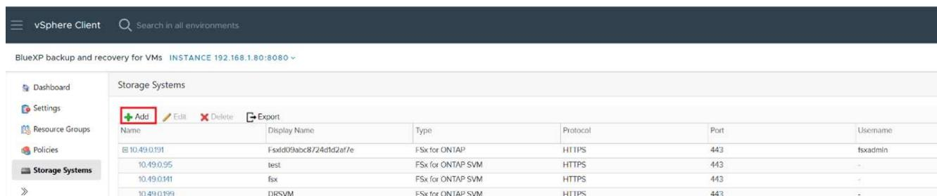
The screenshot shows the vSphere Client interface with the 'Storage Systems' tab selected. A red box highlights the '+ Add' button in the top navigation bar. Below the header, there is a table with columns: Name, Display Name, Type, Protocol, Port, and Username. Five rows are listed:
