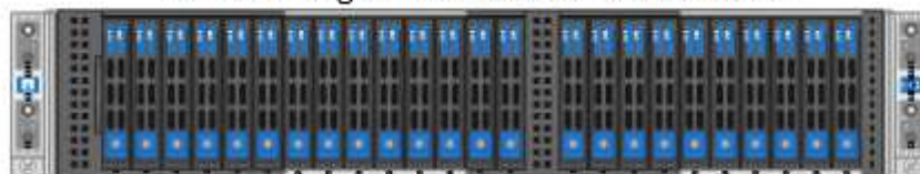
H410S storage nodes in a four-node chassis
