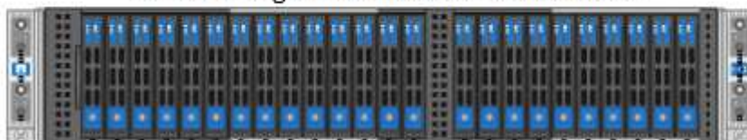
H410S storage nodes in a four-node chassis
