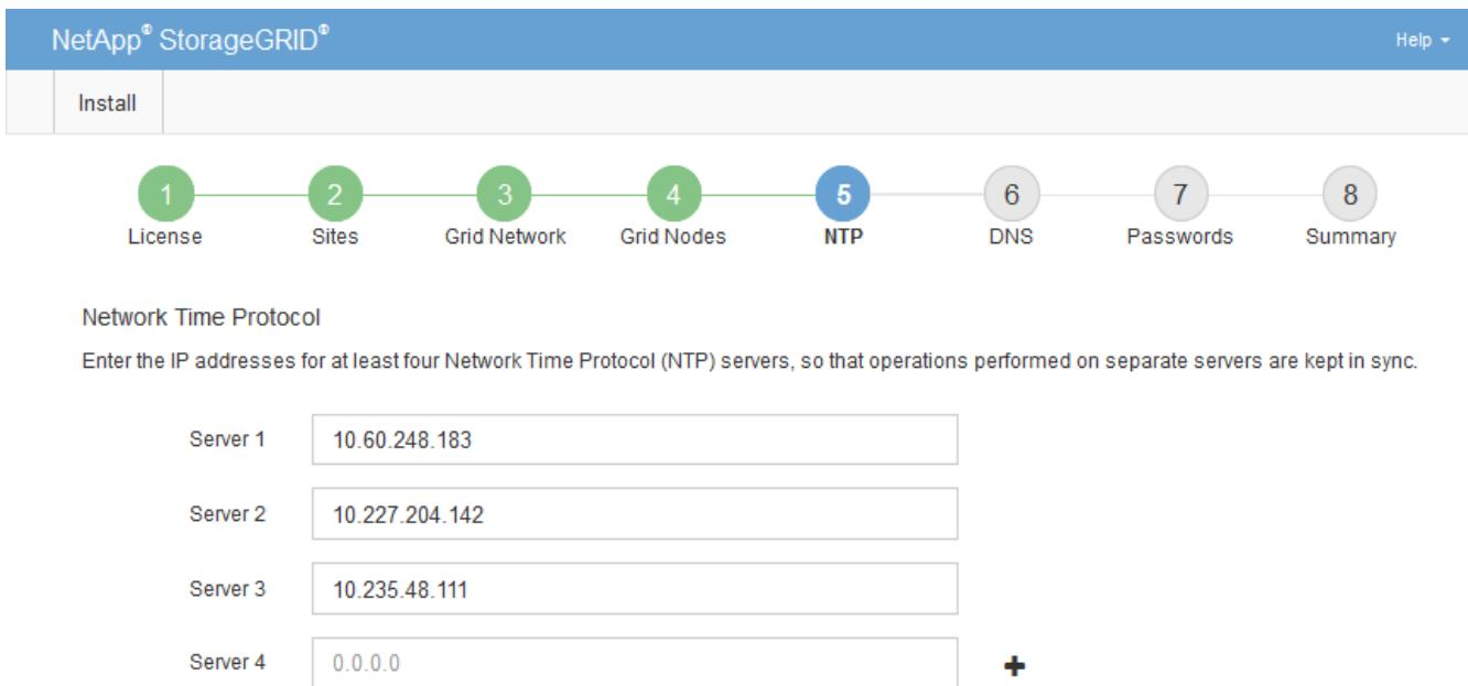
The screenshot shows the NetApp StorageGRID setup wizard at step 5, titled "NTP". The wizard has 8 steps in total: License, Sites, Grid Network, Grid Nodes, NTP, DNS, Passwords, and Summary. Step 5 is highlighted in blue. The "NTP" section asks for IP addresses for at least four NTP servers. It shows four entries: Server 1 (10.60.248.183), Server 2 (10.227.204.142), Server 3 (10.235.48.111), and Server 4 (0.0.0.0). A plus sign (+) button is available to add more servers.
