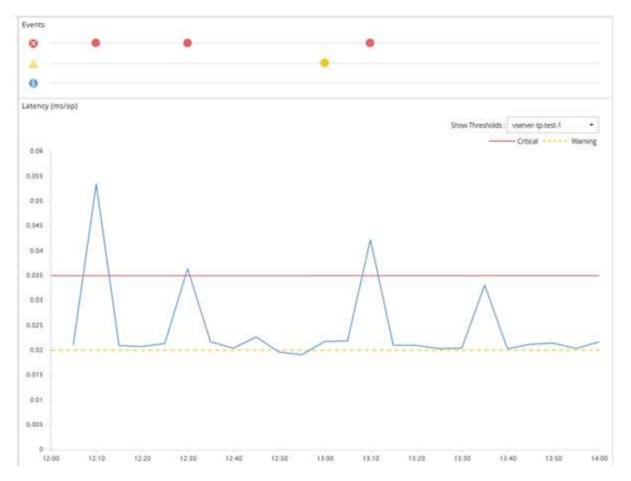
A threshold breach must occur continuously for the specified duration. If the threshold dips below the limit values for any reason, a subsequent breach is considered the start of a new duration.
