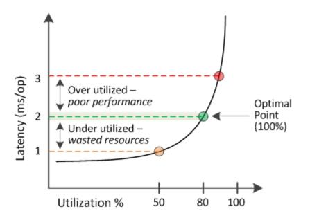
• A performance capacity used percentage equal to 100 is at the optimal point.
