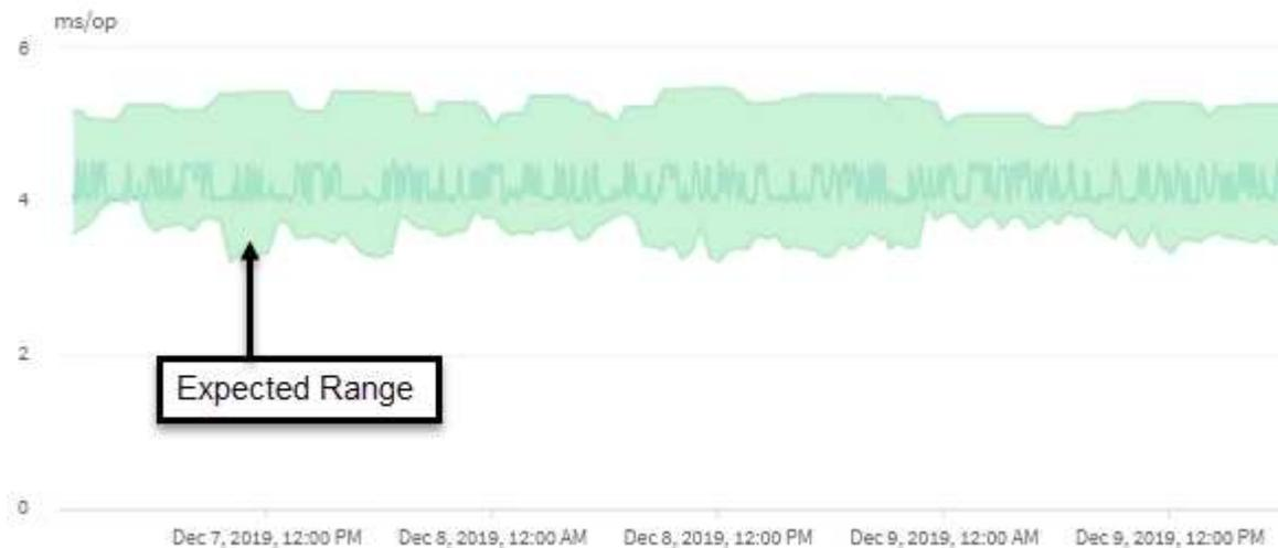
In this example, the latency for a volume has a latency forecast, in gray, of 3.5 milliseconds per operation (ms/op) at its lowest and 5.5 ms/op at its highest. If the actual latency, in blue, suddenly increases to 10 ms/op, due to an intermittent spike in network traffic or contention on a cluster component, it is then above the latency forecast and has exceeded the dynamic performance threshold.
