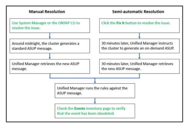
When performing a manual resolution you must log into System Manager or the ONTAP command-line interface to fix the issue. You will be able to verify the issue only after the cluster generates a new AutoSupport message at midnight.
