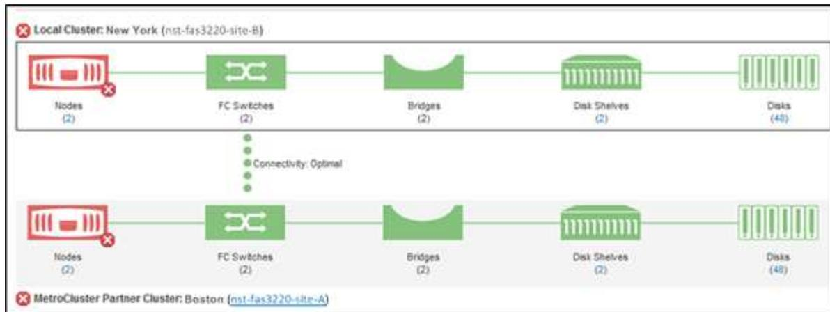
The topology of the MetroCluster configuration is displayed in the corresponding cluster object area. You can use the information displayed in the Cluster / Health details page to rectify any connectivity issues. For example, if the connectivity between the node and the switch in a cluster is down, the following icon is displayed:
