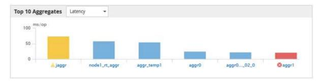
For each graph, the X axis displays the top performers for the selected object type. The Y axis displays units applicable to the selected counter. Clicking the object name link below each vertical bar graph element navigates to the Performance Landing page for the selected object.
