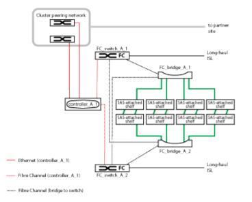
A two-node configuration includes the following connections:
