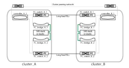
A two-node configuration consists of two clusters, one at each geographically separated site. cluster\_A is located at the first MetroCluster site. cluster\_B is located at the second MetroCluster site. Each site has one SAS storage stack. Additional storage stacks are supported, but only one is shown at each site.
