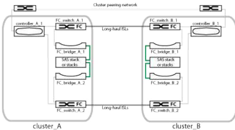
A two-node configuration consists of two clusters, one at each geographically separated site. cluster\_A is located at the first MetroCluster site. cluster\_B is located at the second MetroCluster site. Each site has one SAS storage stack. Additional storage stacks are supported, but only one is shown at each site.
