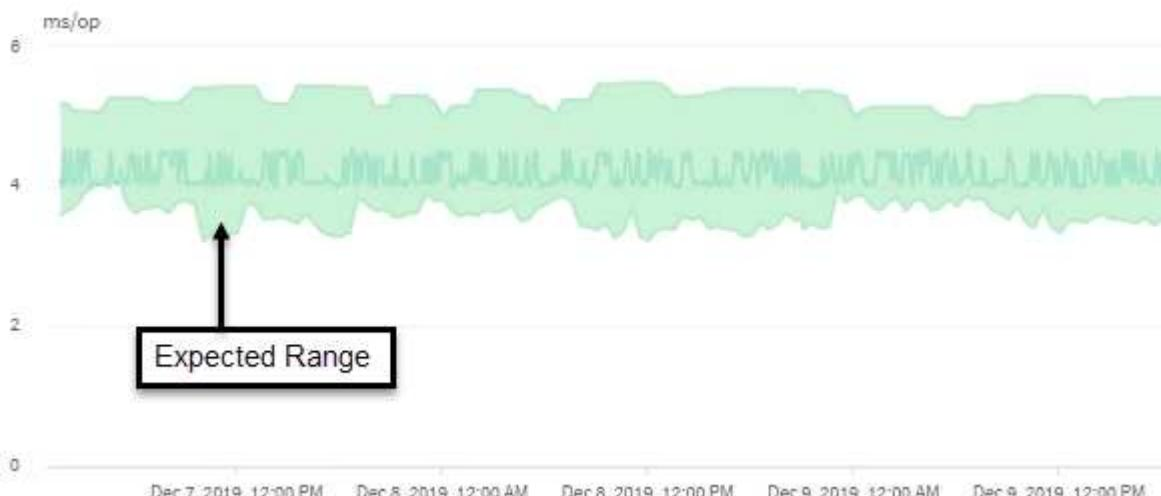
In this example, the latency for a volume has a latency forecast, in gray, of 3.5 milliseconds per operation
