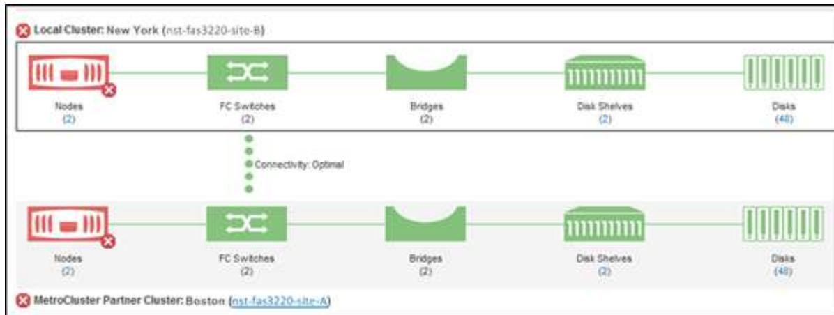
The topology of the MetroCluster configuration is displayed in the corresponding cluster object area. You can use the information displayed in the Cluster / Health details page to rectify any connectivity issues. For example, if the connectivity between the node and the switch in a cluster is down, the following icon is displayed:
