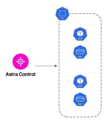
• An individual application deployed within one or more namespaces (helm3 is used in this example)
