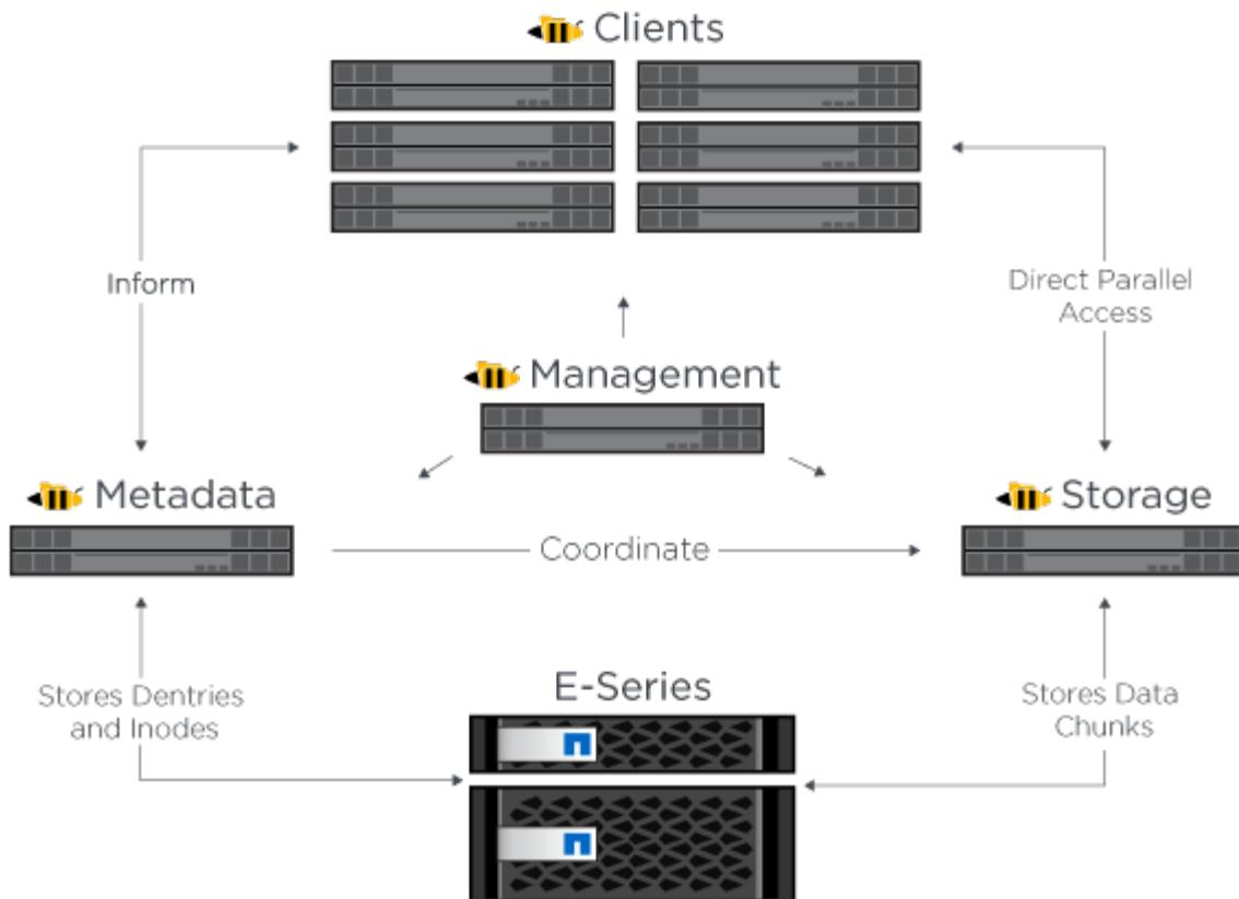
As a parallel file system, BeeGFS stripes its files over multiple server nodes to maximize read/write performance and scalability. The server nodes work together to deliver a single file system that can be simultaneously mounted and accessed by other server nodes, commonly known as *clients*. These clients can see and consume the distributed file system similarly to a local file system such as NTFS, XFS, or ext4.
