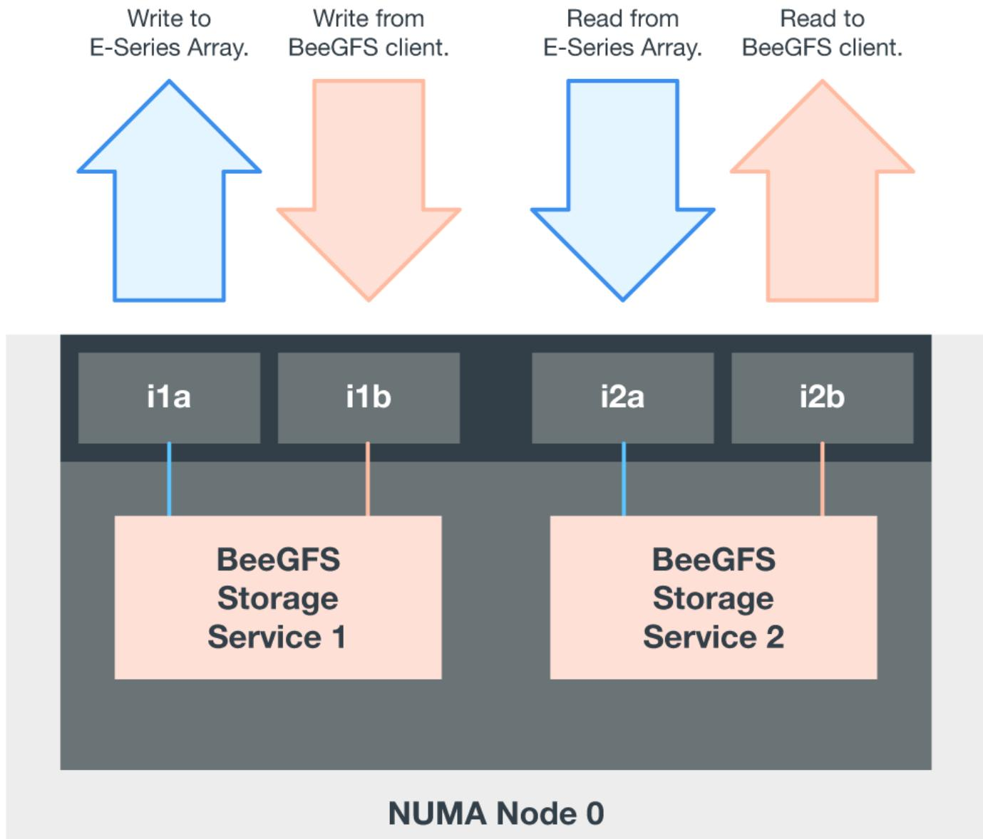
For each BeeGFS service, use the same adapter to connect the preferred port used for client traffic with the path to the block nodes controller that is the primary owner of that service's volumes. For more information, see [Software configuration](#).
