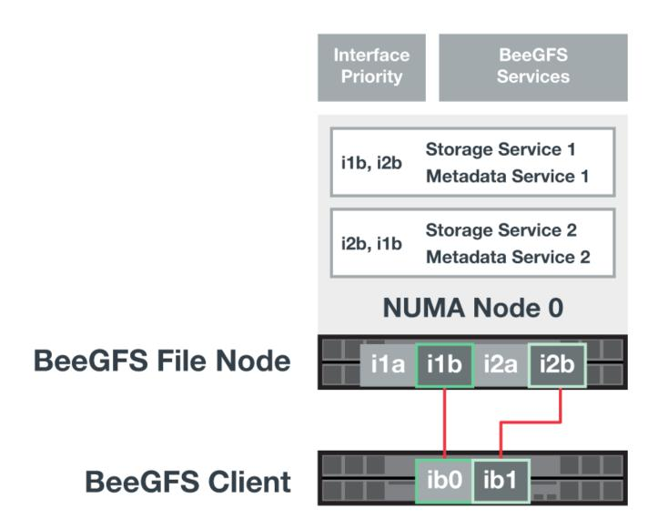
Because each file in BeeGFS is typically striped across multiple storage services, the multi-rail configuration allows the client to achieve more throughput than is possible with a single InfiniBand port. For example, the following code sample shows a common file-striping configuration that allows the client to balance traffic across both interfaces:
