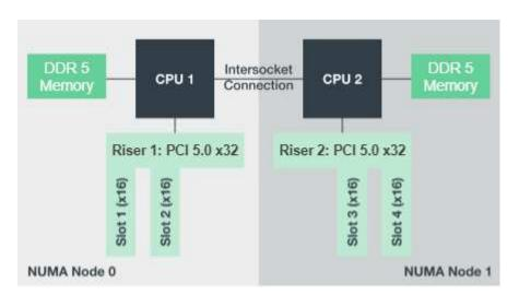
The BeeGFS processes are pinned to a particular NUMA zone to ensure that the interfaces used are in the same zone. This configuration avoids the need for remote access over the inter-socket connection. The inter-socket connection is sometimes known as the QPI or GMI2 link; even in modern processor architectures, they can be a bottleneck when using high-speed networking like HDR InfiniBand.
