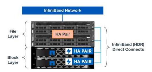
The BeeGFS on NetApp solution runs across all building blocks in the deployment. The first building block
