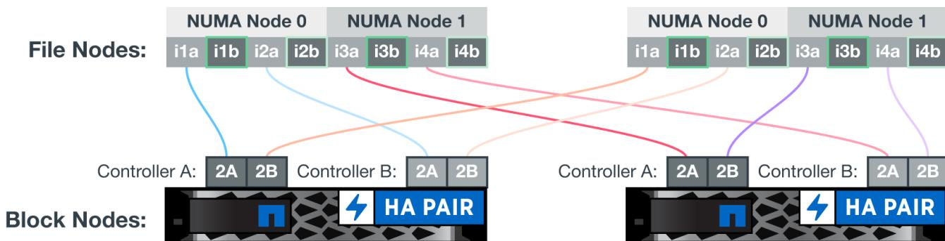
When using splitter cables to connect the storage switch to file nodes, one cable should branch out and connect to the ports outlined in light green. Another cable should branch out and connect to the ports outlined in dark green.
