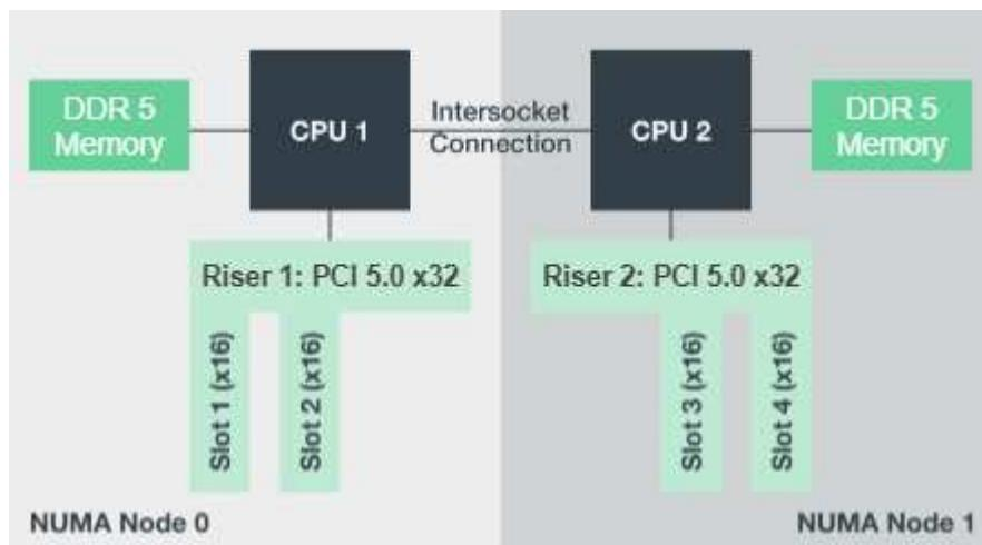
The BeeGFS processes are pinned to a particular NUMA zone to ensure that the interfaces used are in the same zone. This configuration avoids the need for remote access over the inter-socket connection. The inter-socket connection is sometimes known as the QPI or GMI2 link; even in modern processor architectures, they can be a bottleneck when using high-speed networking like HDR InfiniBand.
