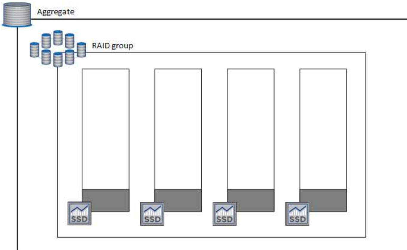
When the Console creates an aggregate, it starts with one RAID group. If additional capacity is needed, it grows the aggregate by increasing the capacity of all disks in the RAID group by the same amount. The capacity increase is either a minimum of 256 GiB or 10% of the aggregate's size.
