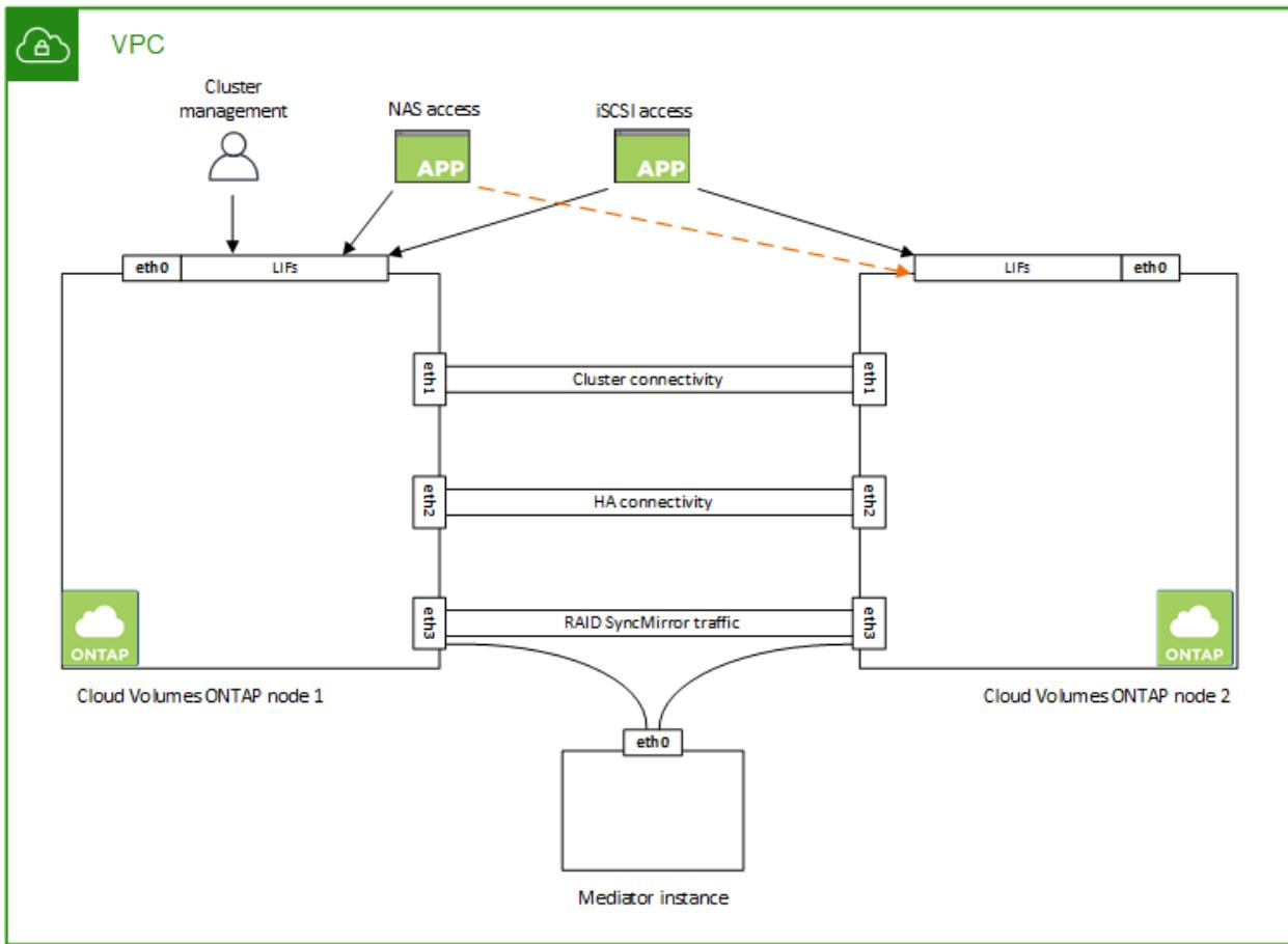
The number of private IP addresses required for an HA pair depends on which deployment model you choose. An HA pair deployed in a *single* AWS Availability Zone (AZ) requires 15 private IP addresses, while an HA pair deployed in *multiple* AZs requires 13 private IP addresses.
