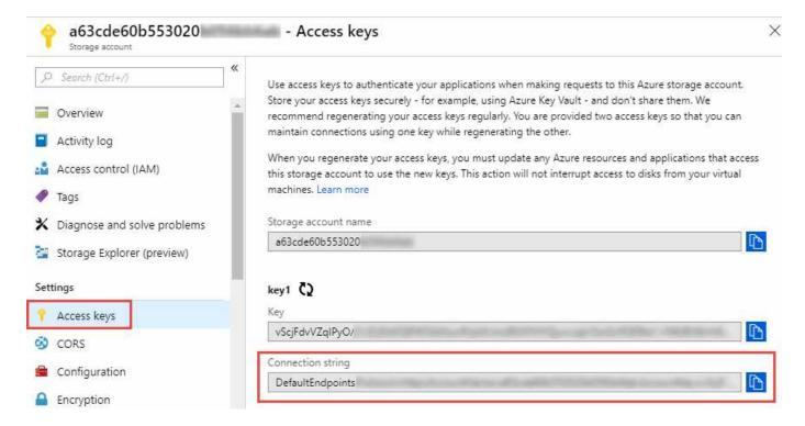
If you want to sync data between two Azure Blob containers, then the connection string must include a shared access signature (SAS). You also have the option to use a SAS when syncing between a Blob container and an NFS or SMB server.
