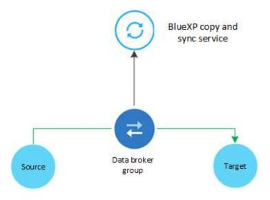
The NetApp data broker software syncs data from a source to a target (this is called a *sync relationship*). You can run the data broker in AWS, Azure, Google Cloud Platform, or on your premises. A data broker group, which consists of one or more data brokers, needs an outbound internet connection over port 443 so it can communicate with the BlueXP copy and sync service and contact a few other services and repositories. View the list of endpoints.
