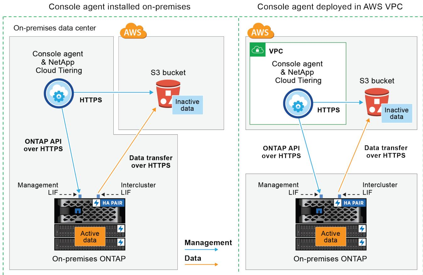
The following diagram shows the **private connection** method and the connections that you need to prepare between the components. You can use the Console agent that you've installed on your premises, or an agent that you've deployed in the AWS VPC.
