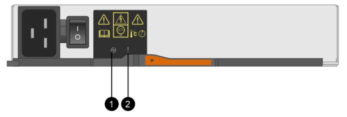
(1) *Power LED*. If it is **Solid green**, the power canister is functioning correctly. If it is **Off**, the power canister failed, the AC switch is turned off, the AC power cord is not properly installed, or the AC power cord input voltage is not within margin (there is a problem at the source end of the AC power cord).
