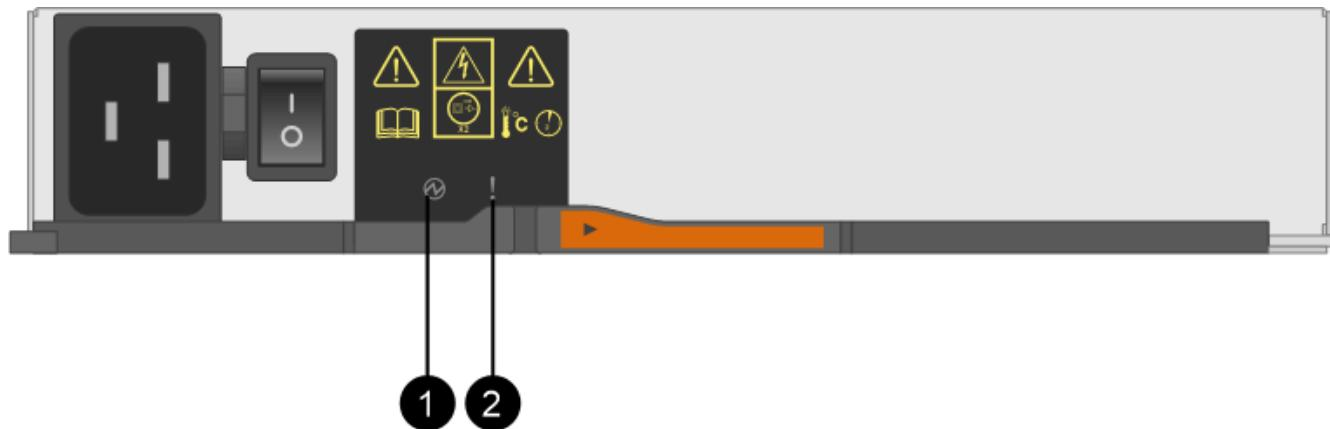
**(1) Power LED.** If it is **Solid green**, the power canister is functioning correctly. If it is **Off**, the power canister failed, the AC switch is turned off, the AC power cord is not properly installed, or the AC power cord input voltage is not within margin (there is a problem at the source end of the AC power cord).
