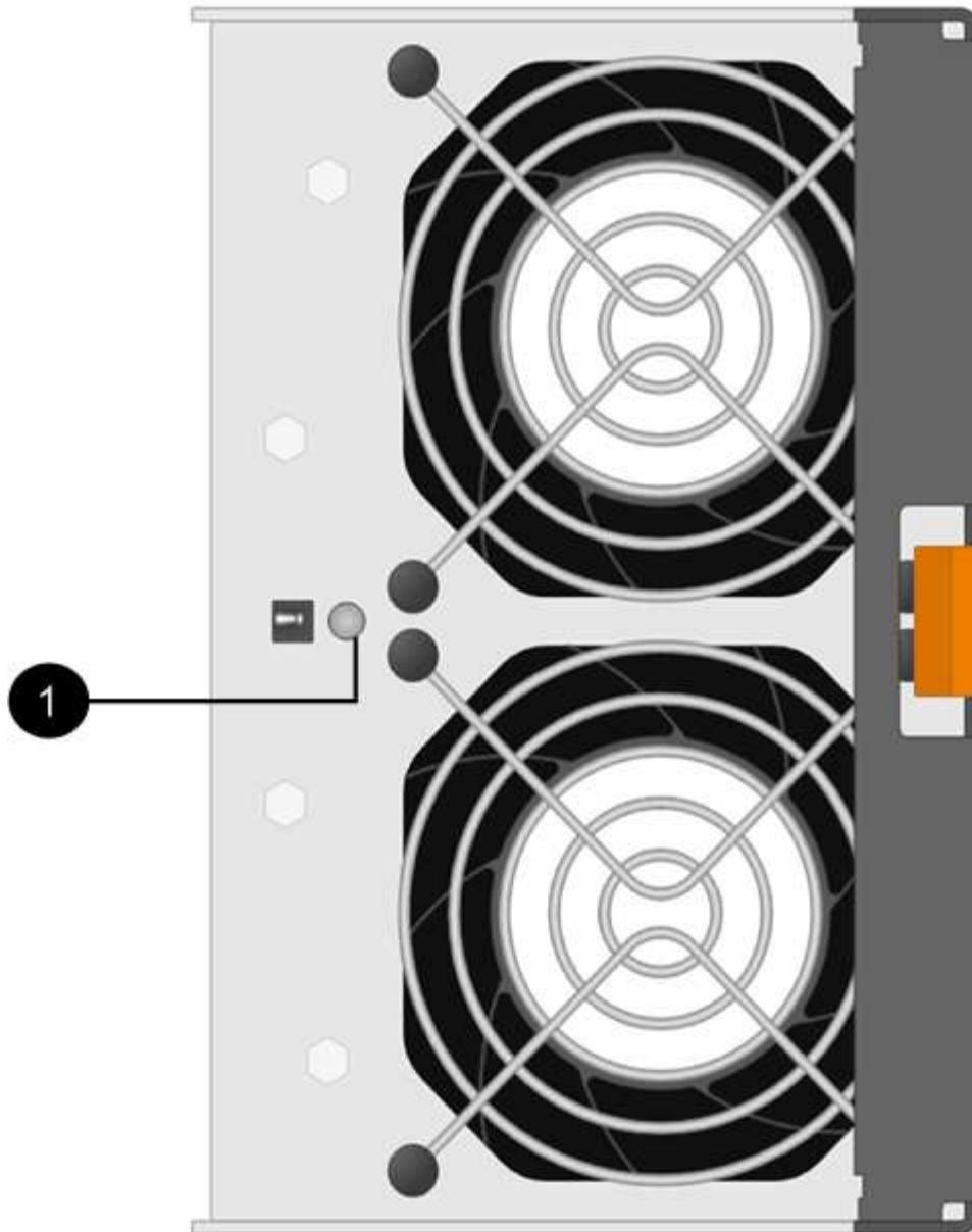
(1) *Attention LED*. If this LED displays as **Solid amber**, then the fan has a fault.
