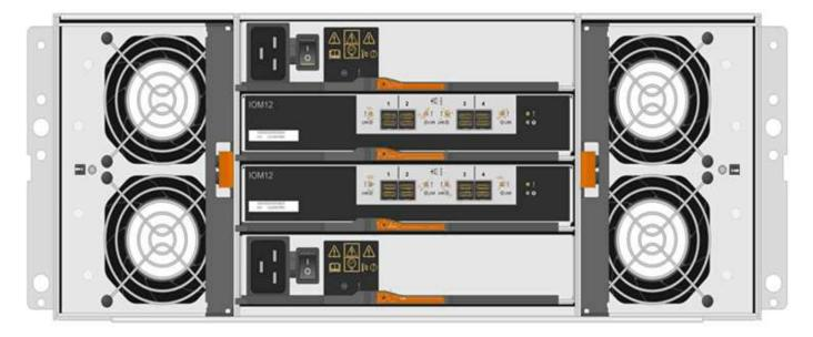
**Possible equipment damage** — If you replace a fan canister with the power turned on, you must complete the replacement procedure within 30 minutes to prevent the possibility of overheating the equipment.
