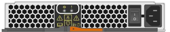
If the Power LED is **solid green**, the power supply is functioning correctly. If it is **Off**, the power supply failed, the AC switch is turned off, the AC power cord is not properly installed, or the AC power cord input voltage is not within margin (there is a problem at the source end of the AC power cord).
