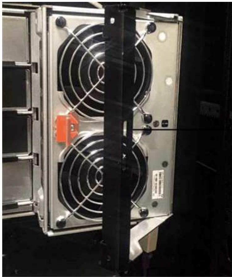
**(1) Handle to pull the fan canister out.**
