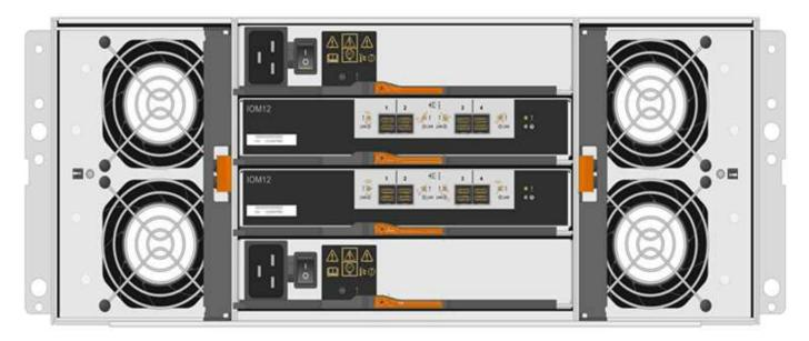
The following figure shows a power canister:
