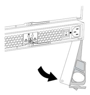
4. Use the cam handle to slide the power supply out of the system.
