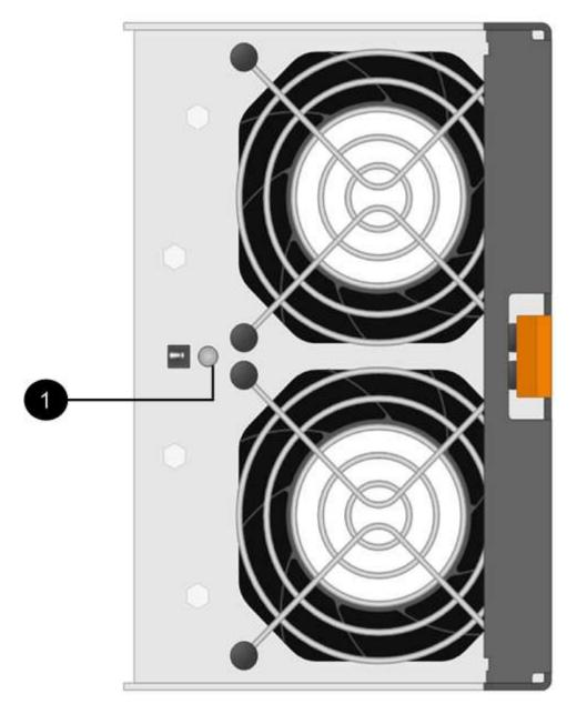
(1) Attention LED. If this LED displays as Solid amber, then the fan has a fault.
