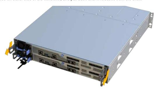
6. Using two hands and the handles, slide the controller canister out of the shelf. When the front of the
