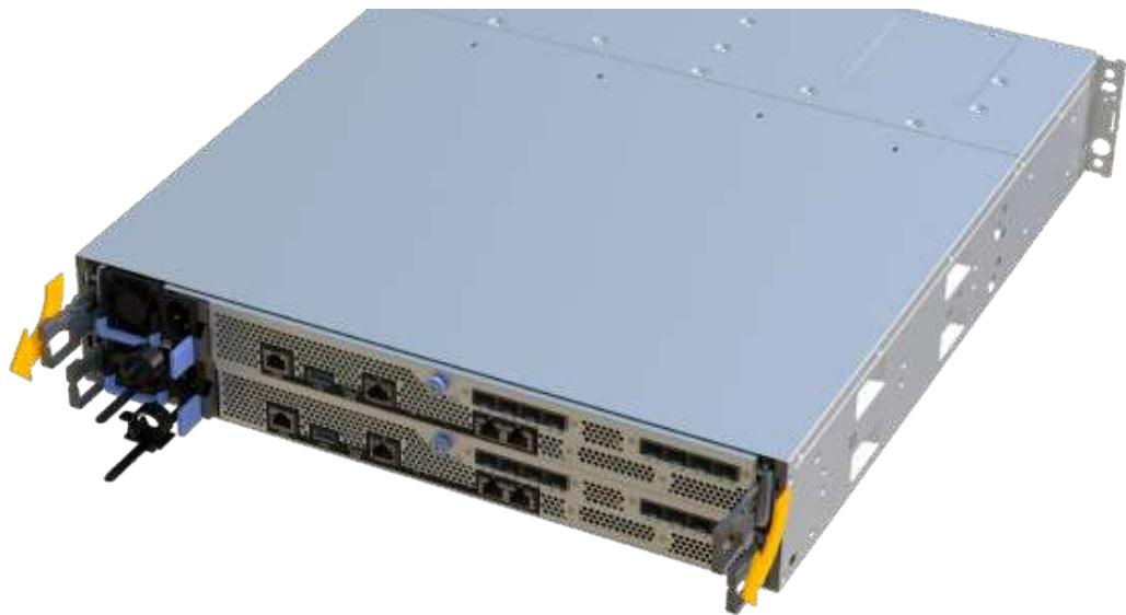
6. Using two hands and the handles, slide the controller canister out of the shelf. When the front of the controller is free of the enclosure, use two hands to pull it out completely.
