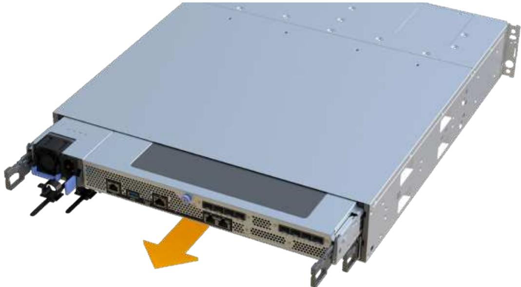
7. Place the controller canister on a flat, static-free surface.
