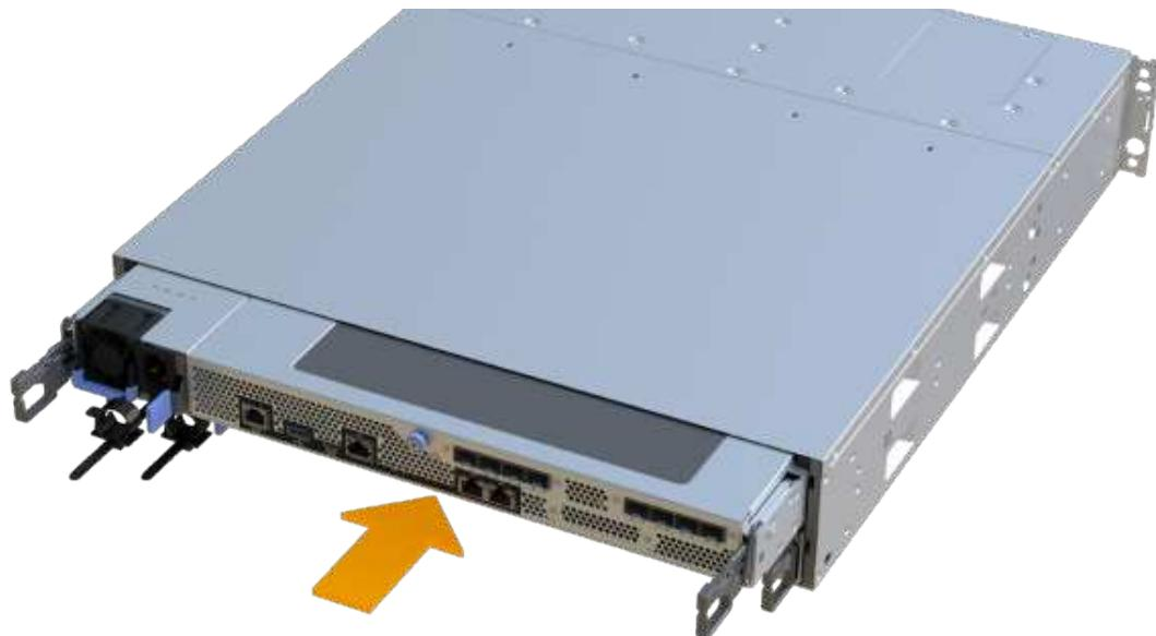
3. Install the SFPs into the new HIC and reconnect all the cables.
