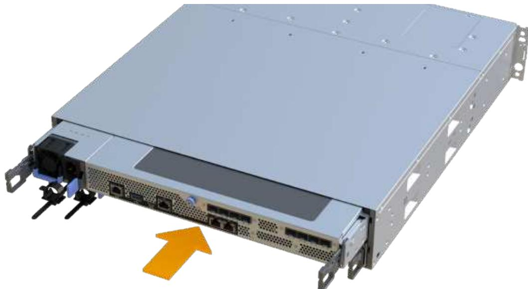
3. If removed, install the SFPs into the new HIC and reconnect all the cables. If you are using more than one host protocol, be sure to install the SFPs in the correct host ports.
