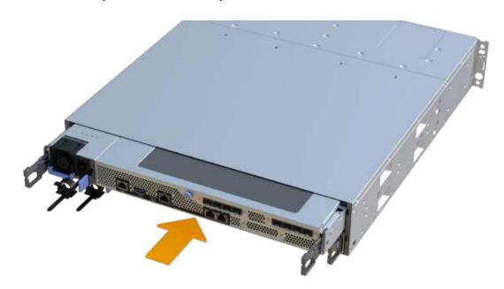
3. If removed, install the SFPs into the new HIC and reconnect all the cables. If you are using more than one host protocol, be sure to install the SFPs in the correct host ports.
