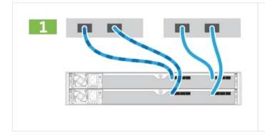
1. Connect each host adapter directly to the host ports on the controllers.
