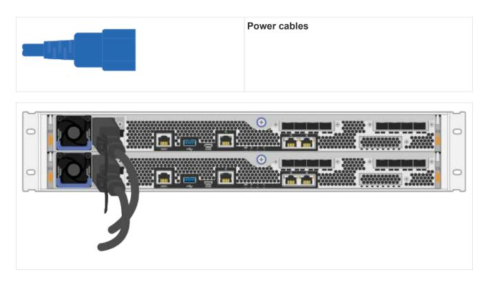
2. Connect the two power cables, one from each controller, to two separate power distribution units (PDUs) in the cabinet or rack.
