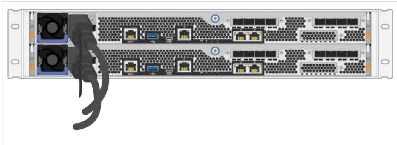
2. Connect the two power cables, one from each controller, to two separate power distribution units (PDUs) in the cabinet or rack.
