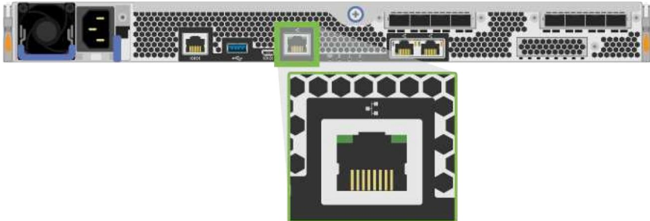
2. Open a browser and connect to the storage system using one of the controller IP addresses provided to you by your network administrator.
